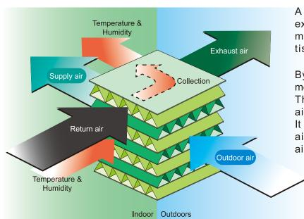
A total heat(temperature and humidity) exchange element with special thin paper membrane, that is made with our unique tissue papermaking technology.
